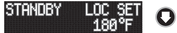
Figure 22 HeatNet display during Standby (no call for heat) — pressing the DOWN key on the keypad changes the display as shown
